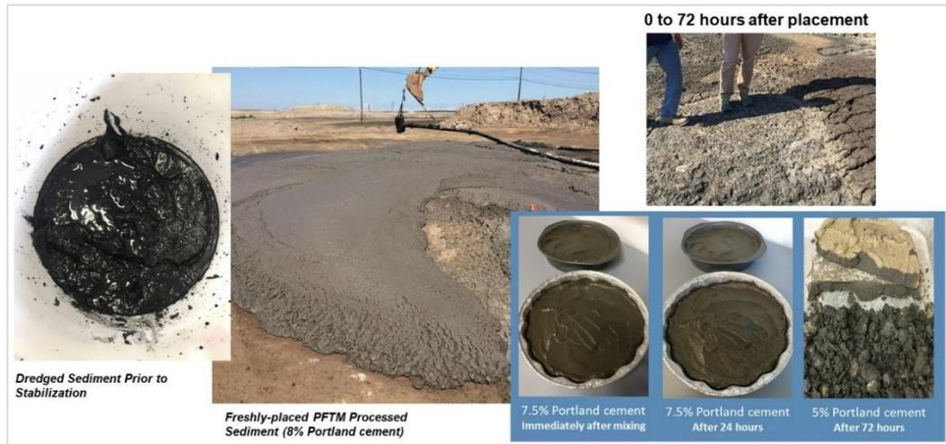
Figure 3-25 Processed sediment using PFTM
