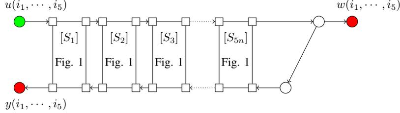
Fig. 2: 5D Generalized IIR lattice digital filter structure. Each square is a copy of the single section of Fig. 1.
