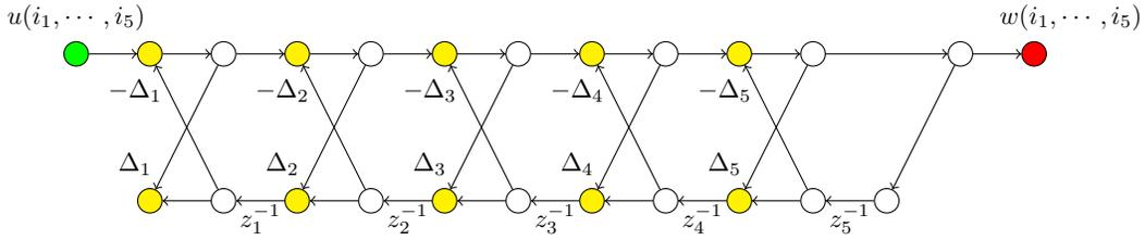
Fig. 3: 5D first-order all-pole digital lattice filter.
