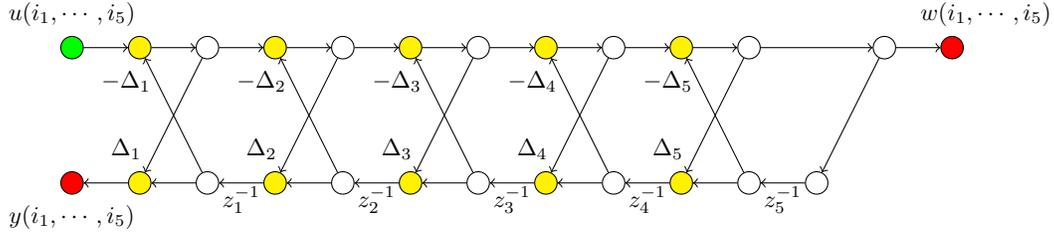
Fig. 1:  $[S_i]$ : 5D first-order IIR digital lattice filter.
