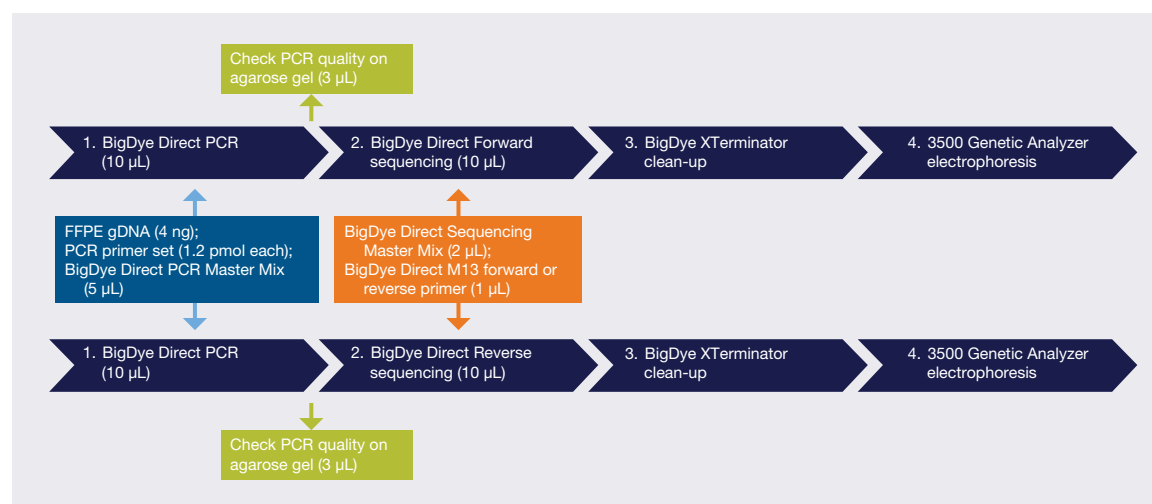
Figure 28. Workflow for BigDye Direct cycle sequencing.
